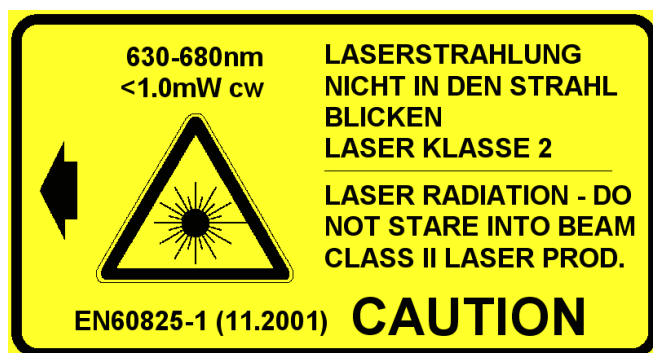
Fig. 5.2 Laser warning label affixed to the pyrometer
