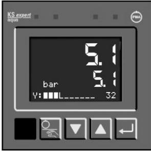
Display of process pressure, setpoint, and output value. Control via Pump 1, setpoint adjustment via ▲ and ▼.
