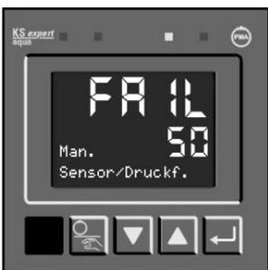
Signal for sensor fault. Output value goes to 50% and can be changed via front-panel keys (emergency operation).
